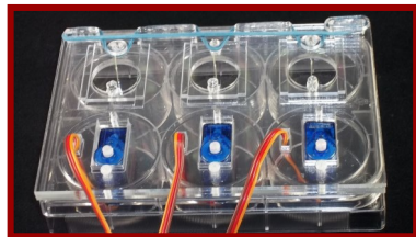
Self-contained medium-throughput I-wire modules, with camera readout on an incubator shelf
