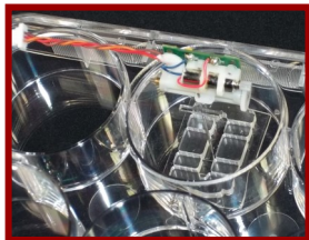
Self-contained medium-throughput I-wire modules, with camera readout on an incubator shelf
