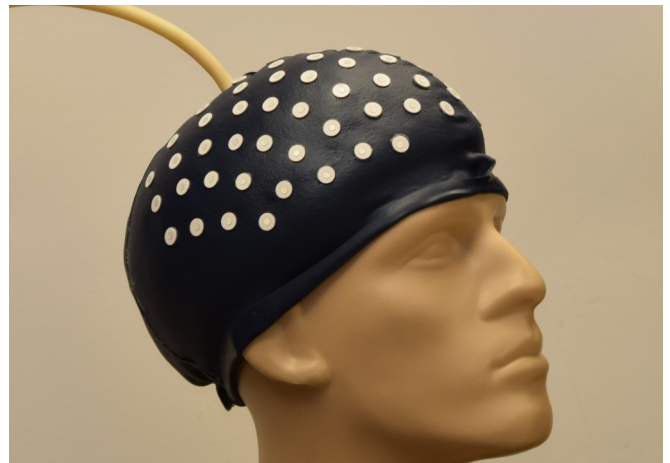
Figure 1: The device creates a rigid, non-slip connection between the patient and an optical tracking marker for use in image-guided surgery.
