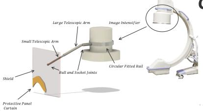
A virtual prototype of the user-friendly shield mount system that attaches around the fluoroscopy machine's image intensifier for seamless integration. The unique 2-arm telescoping system is designed to avoid "kinking" of the arms that may limit positioning abilities and potentially clash with surrounding equipment in the crowded procedural room. The upper arm of the shield is attached to the image intensifier using a smooth rail system to allow for quick and precisely tunable shield movement.
