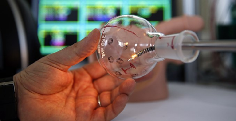
Fig. 1: The image above depicts the robotic platform's capabilities in terms of dexterity and flexibility. A flask is used as a proxy for the bladder to demonstrate the robot's ability to maneuver to and interact with the curved walls.
